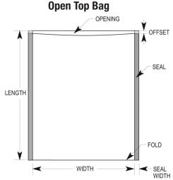
Tolerance (inches): Width -0, +0.250 Length +/- 0.125 Offset 0 to 0.250 Seal width +/- 0.125
